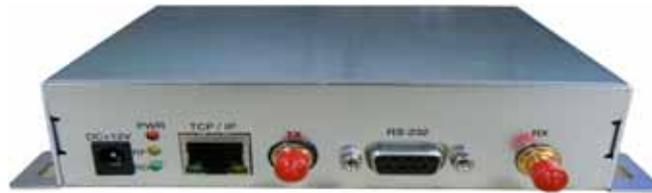
Connected the reader with PC through RS232 or RJ45 Port.
